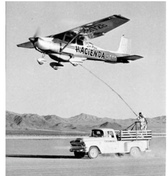
Cessna 172 modified for endurance record flight, refuels from truck
